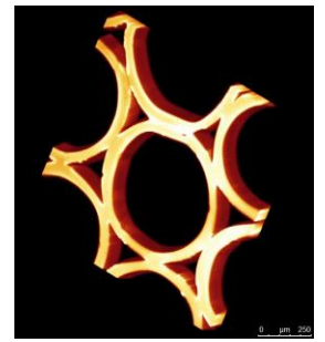
Mesoporous glass bounds visualized by adsorption of fluorescent polyelectrolytes (Surflay)
